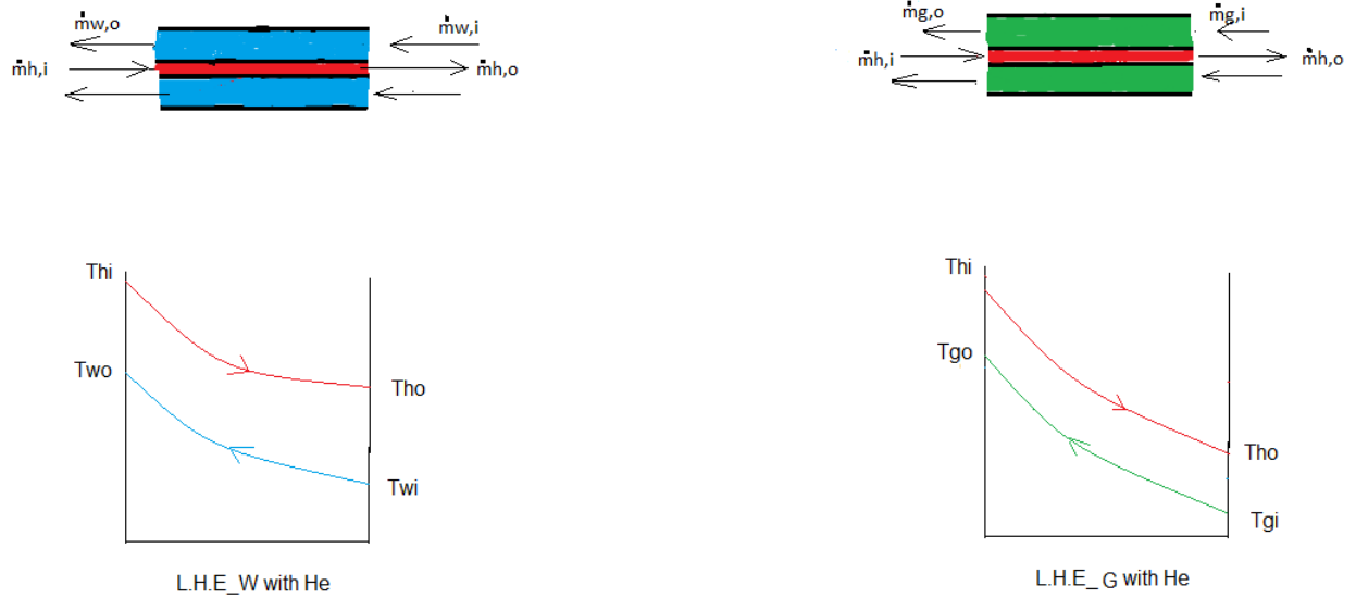
Fig(12):Heat Exchanger Counter Flow two Stage Lift Water with Helium and Right Glycol with Helium (3T)and(5T).
