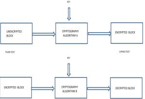
Figure 2: Basic Concept for Symmetric Cryptography
